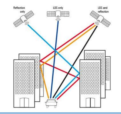
Multiple frequencies remove ionospheric errors and mitigate multipath reflections
